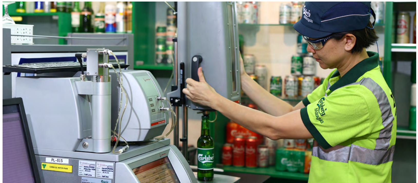
A quality control process being undertaken to test alcohol quality, where testing is conducted on alcohol percentage, CO 2 levels, degree of fermentation and °P (Plato gravity scale).
